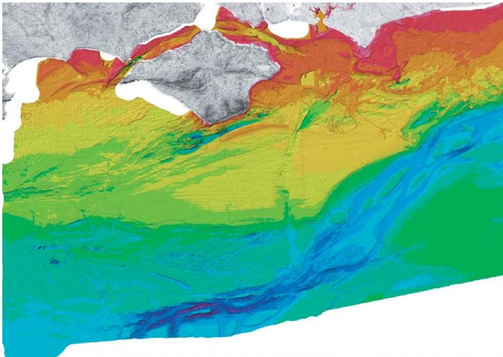
Bathymetry of English Channel south of the Isle of Wight: increasing depth shown by red to blue rainbow scale. Note clear evidence for massive scouring shown by braided channels on the seabed of the deepest part. (Credit: Gupta *et al* 2007; Fig. 2)
