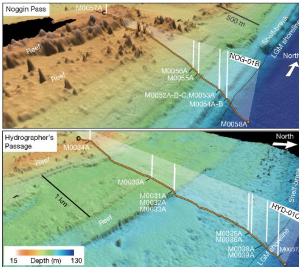
High-resolution sonar images of the sea floor at two sites on the eastern edge of Australia's Great Barrier Reef. They show terraces associated with, the lowest of which corresponds to the Last Glacial Maximum. (Credit: Yokoyama et al. 2018, Figure 1)
